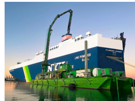
Image of exhaust gas recovery and treatment using emissions capture and control technology
