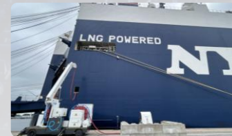
Shore power being supplied to an NYK-operated LNG-fueled vehicle carrier
