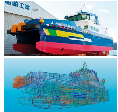
Crew transfer vessel Comparison of actual ship photo (top) and 3D model (bottom)
