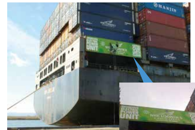
A containership receiving electricity from shore
