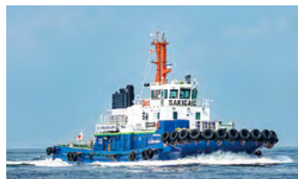
Sakigake, ammonia-fueled tugboat converted from LNG-fueled predecessor
