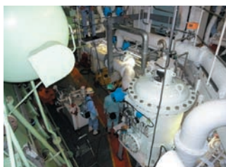
Seawater filter in the ballast water system
